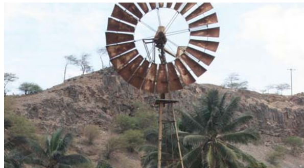
Windmill water pumping, Cape Verde
