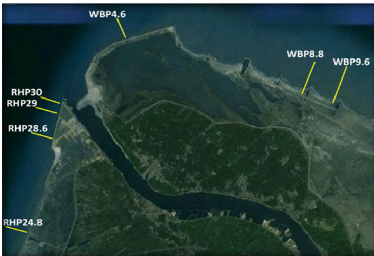
Fig. 4 Location of the selected profiles along eastern and western sides of Rosetta outlet used in calibration and sensitivity analysis
